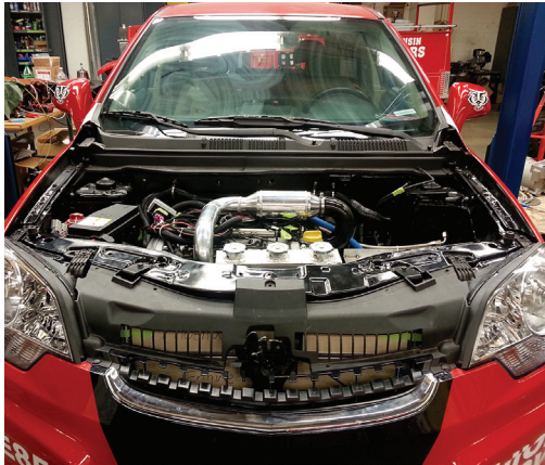
L: On-board generator for the hybrid vehicle with Engine Research Center RCCI-modified engine installed in the engine bay. Middle: A close-up view of the cutting-edge engine assembly. R: The same hybrid vehicle, parked in front of Grainger Hall to generate interest.
